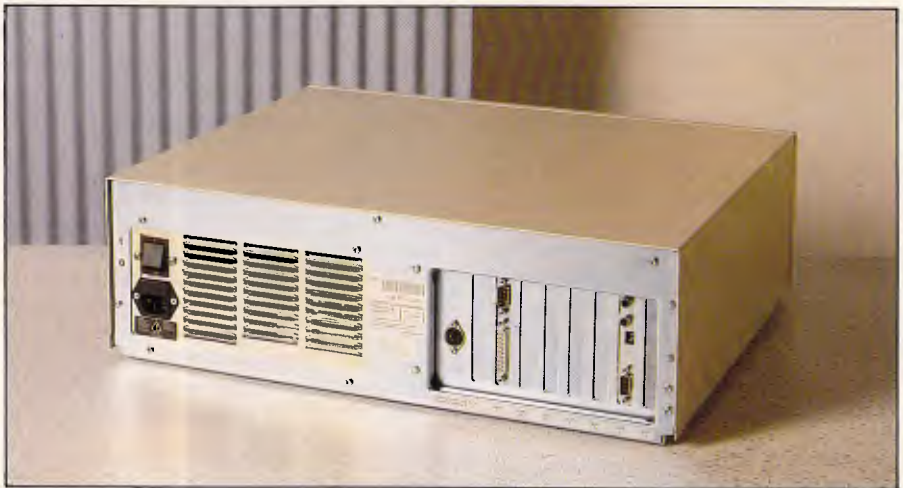
Input/output is via expansion boards, but 32-bit expansion is internal only
